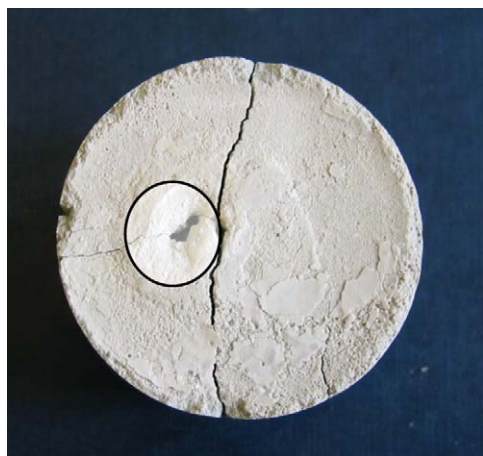
Fig. 6. Hole formed on the top surface of BFS/PC system after 1 day (the cracks were caused by breaking the sample to observe corrosion).
